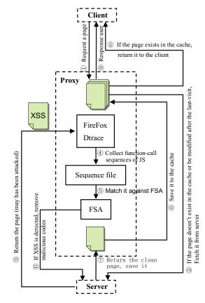
Figure 3. The process of runtime monitoring.
