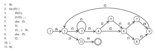
Figure 1. A sample program and its automation learned by FSA-algorithm.
